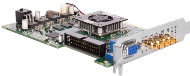
4채널 microEnable 5 marathon VCX-QP / 출처: Silicon Software
