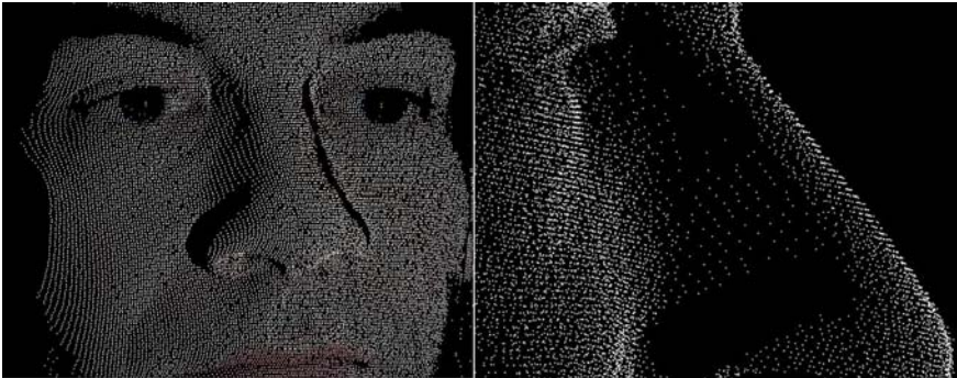
Scan viewed from two angles, taken with Pathfinder laser range scanner
