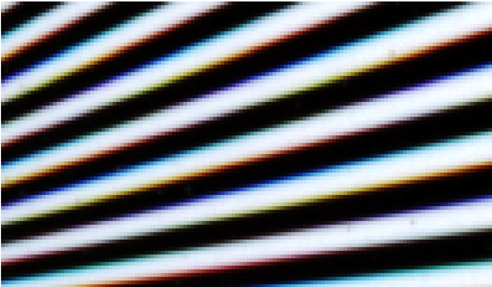
Fig. 4: Edge Artifacts in an Image with an 8:8.318 Aspect Ratio (Colors Enhanced)
